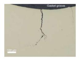
Stress corrosion cracks in one of the V170 plates.
