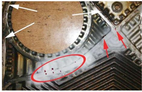
V85 plate. In addition to the obvious and severe corrosion and cracking along the outer gasket groove (marked with arrows), the use of red dye pentrant revealed numerous performations along the gasket diagonal, shown as red spots (highlighted by the red arrows and in the encircled area.)
