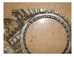
V85 plate. The damages are mainly located in the gasket grooves.
